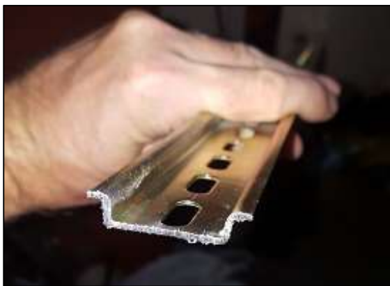
Figure 5: Typical DIN rail
