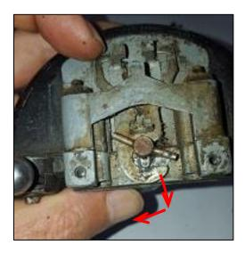
7. Carefully separate the motor base from the semi-circular top.
