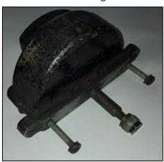
Remove the screws attaching each end of the mounting bracket to the wiper body.Slide the bracket off the shaft.
