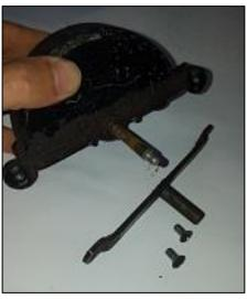
Remove the felt seal and then the metal washer off the shaft.
