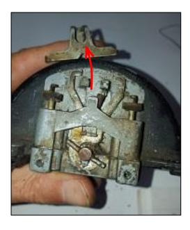
6. Push the rocker reverse bracket down so that it releases from behind the lip on the
