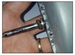
12. Slide the mounting bracket over the shaft and secure with the two screws to the wiper body on either end.
