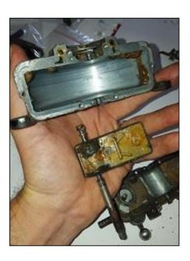
9. Remove the rocker reverse bracket and the spring.
