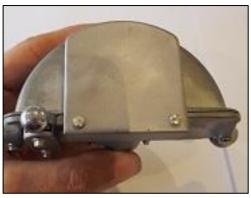
11. Slide the washers onto the shaft – metal washer first, then fibre.
