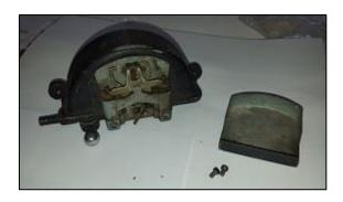
4. Remove the 4 special head screws holding the base to the semi-circular top. These are at the shaft and at the sides. Also remove the 2 slot head screws exposed when the cover plate was removed in Step 3. The longer special head screws go to the sides of the base, not at the shaft.
