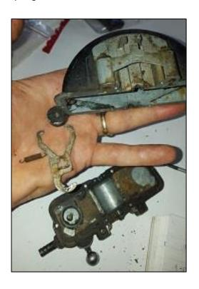
10.Carefully remove the gaskets from the motor body. Yours may be reusable, so do this carefully. A small razor blade or exacto knife may help.
