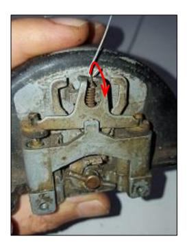
Release the spring. Slide the bracket up, which will bring the brass plungers with it on each side. Unhook the bracket arms from the plungers on each side and slide the bracket forward and out.
