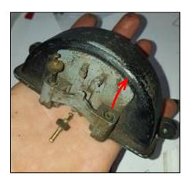
12. Remove the 2 special head screws holding the cover on the control knob and remove the cover.
