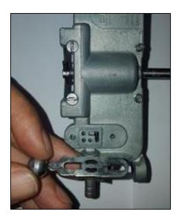
The spring in the cover pushes against the other side of the lever. This can get a slightly heavier grease that will provide more friction protection as there are no channels to block up. Again, I used a light smear of wheel bearing grease. The open end of the spring was originally on the handle side of the lever on mine. I put it back together this way.
